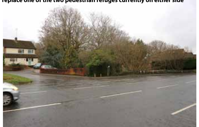
A zebra crossing is proposed to link the Leap Valley path either side of Badminton Road, which would involve building out the pavement where the eastern part of the path meets the road
